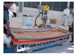
The low net closing pressure and low internal mechanical forces enable use of lightweight tools. For that reason it is possible to use tools similar (or adapted from) open moulding tools without significant extra investment.
