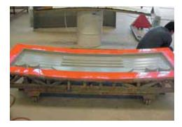
The process requires a rigid female mould and a semi-rigid male top mould. The mould closure occurs by applying vacuum aided by simple clamping mechanisms.
