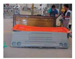
When the reinforcement package is fully impregnated with resin, the resin feed is cut off. Still under vacuum, the laminate is left to cure.
