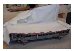
The resin is usually injected at low pressure (max. 1 bar) into a peripheral channel surrounding the part, and vacuum is applied to an exit port near the centre of the part.
